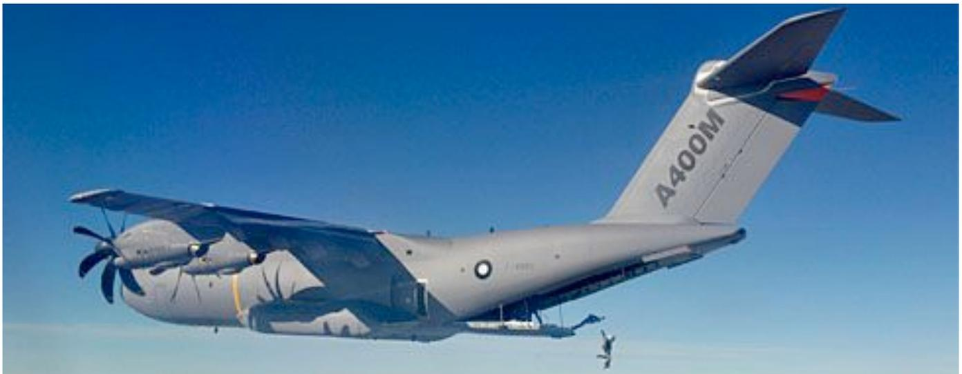
can carry 30 tonnes to a distance of 4,500 km (2,450 nautical miles) or 20 tonnes to a distance of 6,400 km (3,450 nautical miles). Its modular bay can hold a combination of these materials while offering 54 seats for soldiers to be deployed, search and rescue teams, medical support, engineering, etc..
