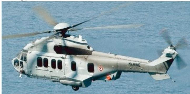
necessary. Equipped with additional tanks, the EC 225 SECMAR is capable of carrying out a rescue of 15 people up to 250 nautical (465 km) from the coast.
